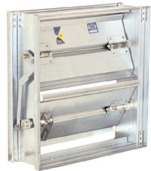
D2 3V Blades, Class 2 Leakage 10cfm/ft2 @ 4 in. wg, Vinyl Blade Seals
