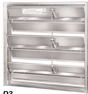
D3 3V Blades, Class 3 Leakage 120cfm/ft2 @ 4 in. wg, No Blade Seals
