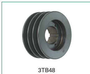
FIXED PITCH, 3 GROOVE, "A" OR "B" BELT, SPLIT TAPER HUB
