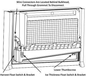
Ice Thickness Float Switch & Bracket
